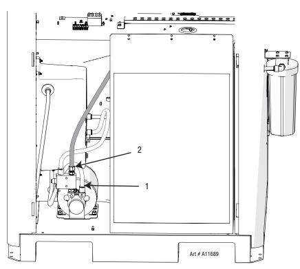
5. Reconnect those two fittings and then remove the filter bowl from the canister at the rear of the power supply. Pour this remaining coolant into the container and replace the filter bowl.
