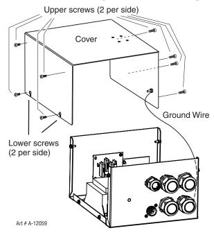
3. The Arc Starter must be grounded; the grounding terminal is marked  $\downarrow$ . Refer to the previous section for grounding details.
