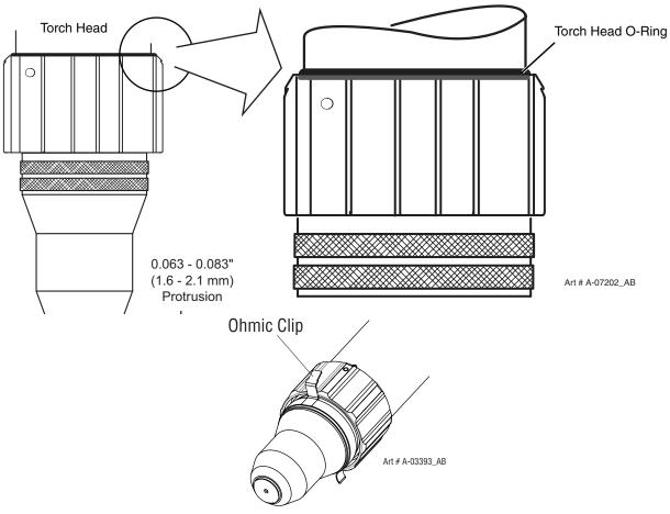
Installing Assembled Cartridge Onto Torch Head
