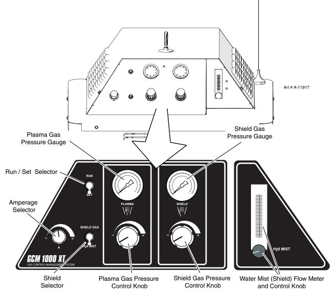
Run / Set Selector: Use SET position to adjust plasma and shield pressures and flows. Once these are set, switch to RUN position for operation.
