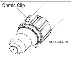
9. Connect the wire lead from the height finder to the ohmic clip if using ohmic torch height sensing.
