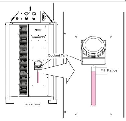
3. After the complete system has been installed, check that the coolant has been pumped through the system as follows (see NOTE):
