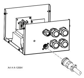
Control Cable from Power Supply rear panel
