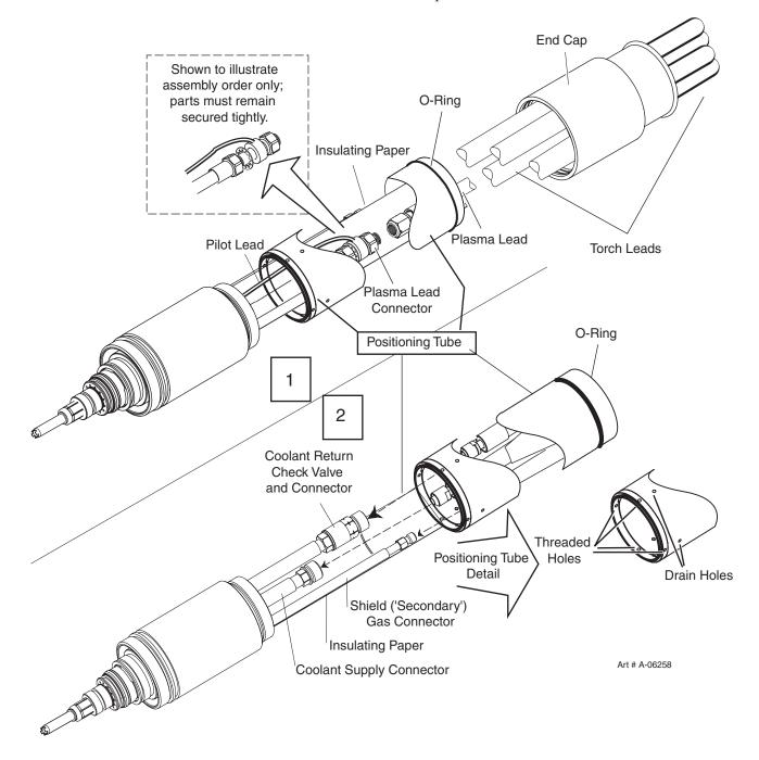
5. Slide the positioning tube down to the torch head. Hold the torch head stationary. Rotate the positioning tube onto the torch head. Pull the leads back as needed to ensure a proper fit through the Mounting Tube. Do not let the torch leads twist.
