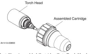
Installing Assembled Cartridge Onto Torch Head
