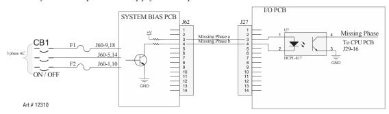
Normally when the phase is not missing the transistor is on which turns on the opto-isolator making the signal "Missing Phase" low.
