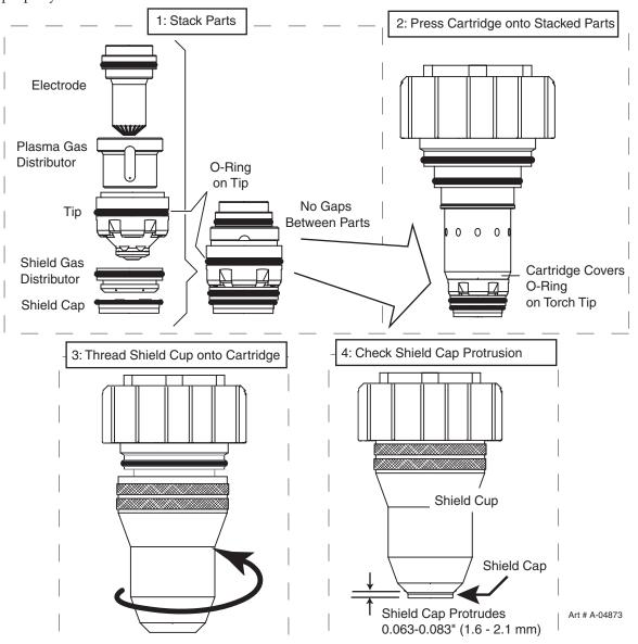
5. Use the removal tool to hold the cartridge assembly, while turning the shield cap onto the cartridge assembly. When this group is fully assembled, the shield should protrude from the front of the shield cup 0.063" to 0.083" (1.6 - 2.1 mm). Without this protrusion the shield cup is not properly tightened onto the cartridge assembly.
