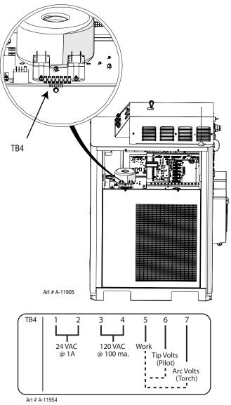
There are holes added in the rear panel for customer wiring. This, rather than the one in the CCM will be the preferred place for customer added wiring (and strain relief) for connections to height controls, etc..
