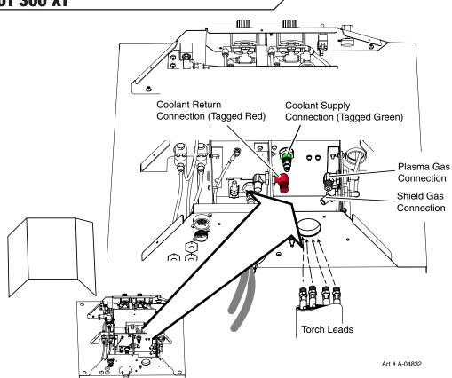
5. Fold the end of the leads outer jacket back over the connection ring inside the module. Slide the leads clamp over the jacket and fasten the clamp and jacket to the connection ring. Re-install the module top cover.
