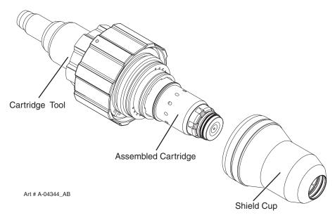
Installing Shield Cup Onto Cartridge
