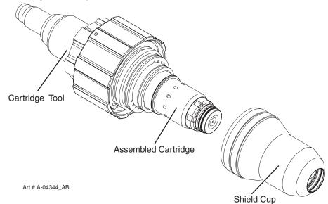
2. Take the Removal Tool off the back of the Cartridge Assembly Use the removal tool to push the consumable parts out of the Cartridge.
