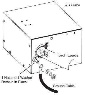
4. Use a clamp to secure the Torch Lead Shield braid brass ring to the port on the Remote Arc Starter as shown.
