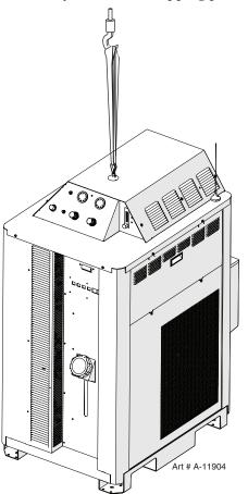
Set the power supply on a solid, level surface. The installer may fasten the power supply to the floor or a supporting fixture with hardware passing through the horizontal parts of the power supply feet.
