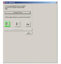
To use the Plate Alignment feature, locate a corner or plate edge and click Set point 1 here. Select which direction the next point is relative to the first location, travel to the second point and click on Confirm point 2 here. This will automatically rotate the program to match the skewed plate
