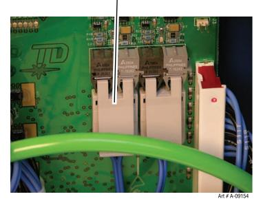
6. Plug the Fiber Optic Cable into the PCB as shown below for the DPC-3000. Make sure the locking tabs are engaged.
