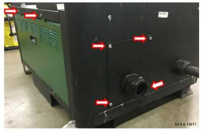
2. Carefully cut back the outer sheath on the primary input power cable to expose the individual wires. Cut back the insulation on the individual wires. Route the power cable through the strain relief and attach the 3 phases to L1, L2, L3 and the green/yellow earth ground wire to ground terminal accessible through the side panel.
