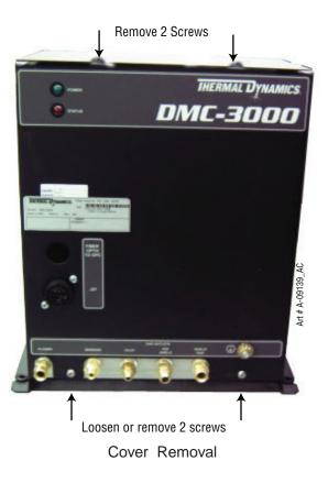
2. Carefully remove the cover from the module noting the attached wire harness that connects to J1. Remove the wire harness and then set the cover to the side.
