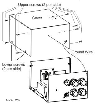
3. The Arc Starter must be grounded; the grounding terminal is marked  $\frac{1}{2}$ . Minimum of 1/0 size wired directly to the star ground. Refer to the previous section for grounding details.
