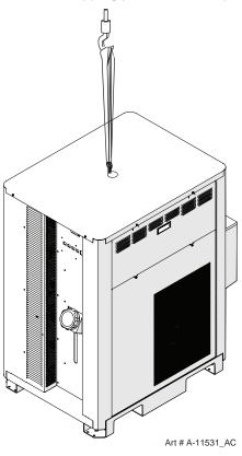
Set the power supply on a solid, level surface. The installer may fasten the power supply to the floor or a supporting fixture with hardware passing through the horizontal parts of the power supply feet.
