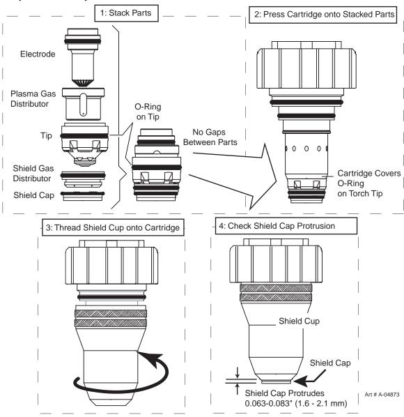
Installing Assembled Cartridge Onto Torch Head
