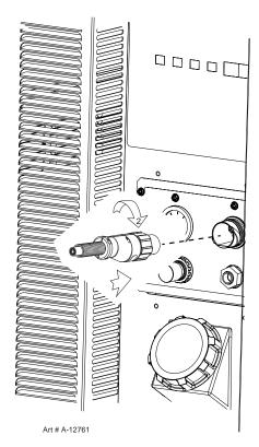
Connecting the Torch to the Power Supply
