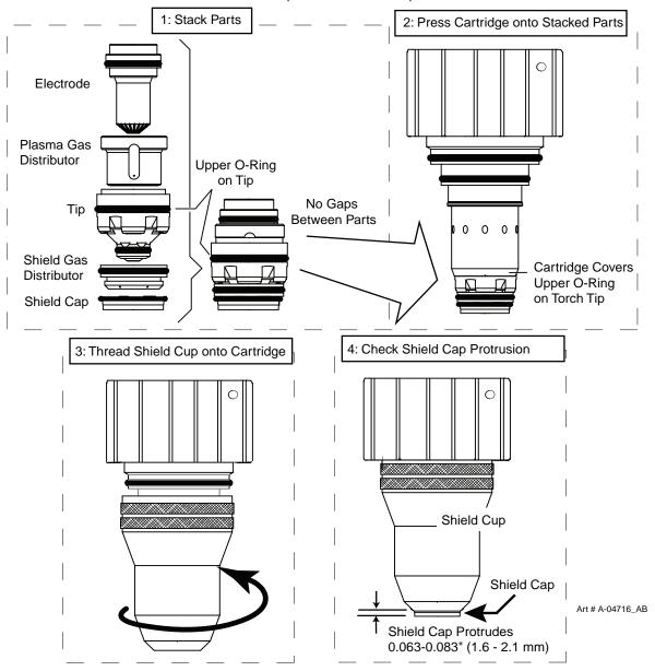
2. Remove the Removal Tool from the Cartridge and install the assembled Cartridge onto the Torch Head.
