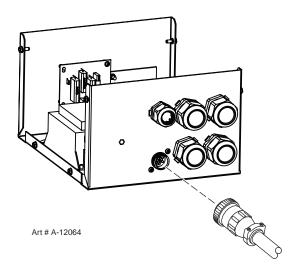
Control Cable from Power Supply rear panel
