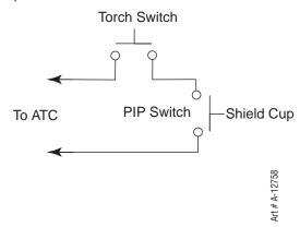
Parts - In - Place Circuit Diagram for Hand Torch
