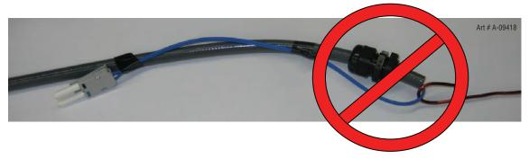
3. Once the fiber cable is installed in the CCM or gas control make sure the strain relief nut is securely tightened onto the hose so the hose can't pull out of it like this:
