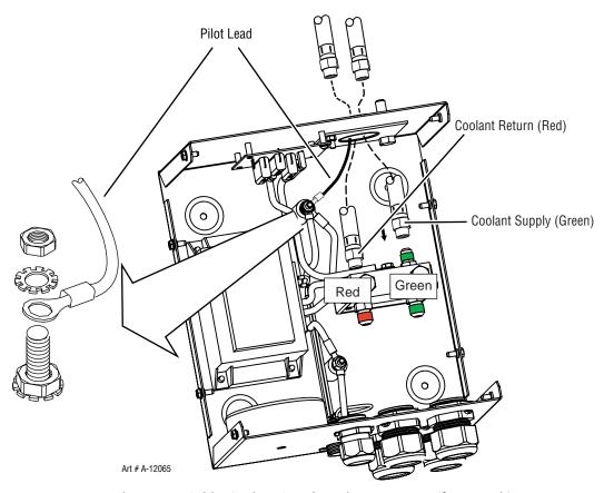
Pilot Return Cable, Coolant Supply and Return Hoses (from Torch)
