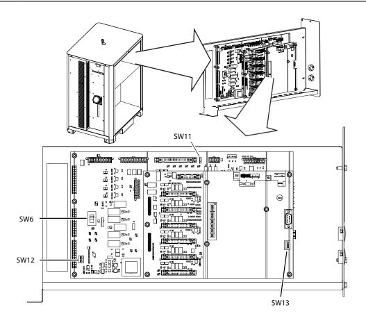
SW-6: OK-to-Move: Contact closure, 120VAC @ 1A (Factory default setting) or DC Volts (16-18vdc@ up to 100 ma.)
