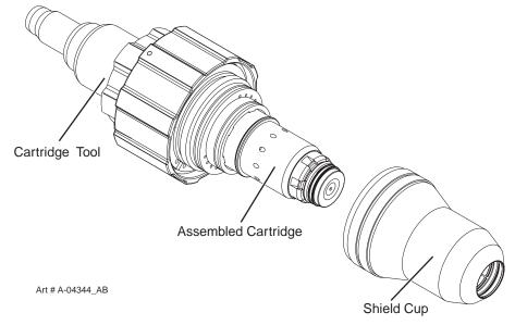
2. Take the Removal Tool off the back of the Cartridge Assembly Use the removal tool to push the consumable parts out of the Cartridge.
