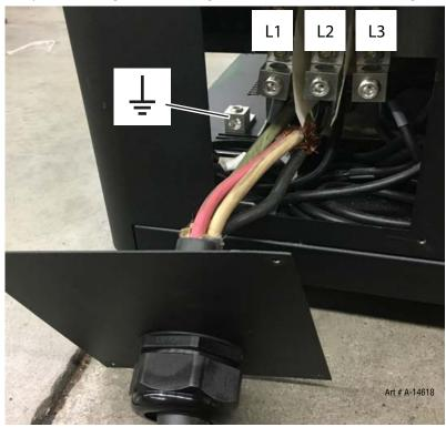
3. Reinstall the access panel and tighten the strain relief around the power cord. Replace the side panel.
