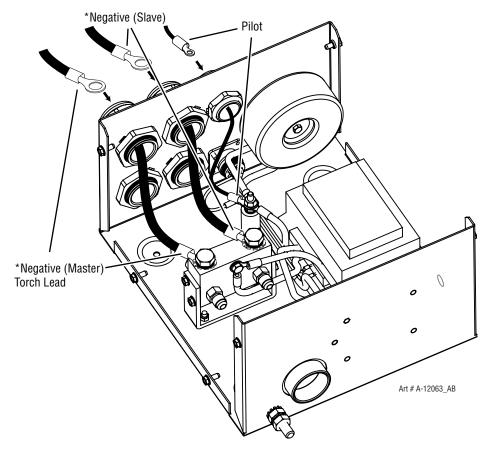
Negative Master, Negative Slave and Pilot Cables (from Power Supply)
