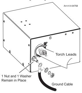
4. Use a clamp to secure the Torch Lead Shield braid brass ring to the port on the Remote Arc Starter as shown.
