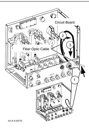
3. Insert the fiber-optic cable connector into the receptacle on the vertically-mounted circuit board as shown. Cable must snap into place.
